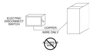
Fig. 28—Disconnect Switch and Furnace
